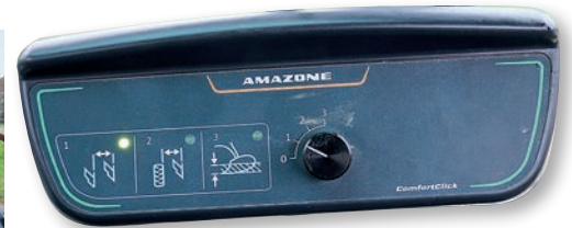
The electro-hydraulic switch box made using the test Teres very simple for novice operators.
