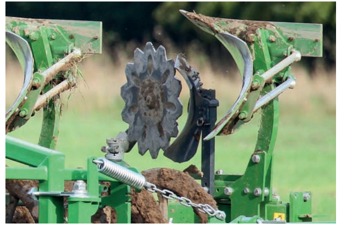
The disc coulters on the last furrow does a neat job. Plain discs and even spring-protected solutions are on the manufacturer's options list.
