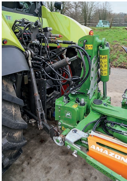
Clutter-free headstock with SmartCenter offers various coupling options to the plough tractor.
