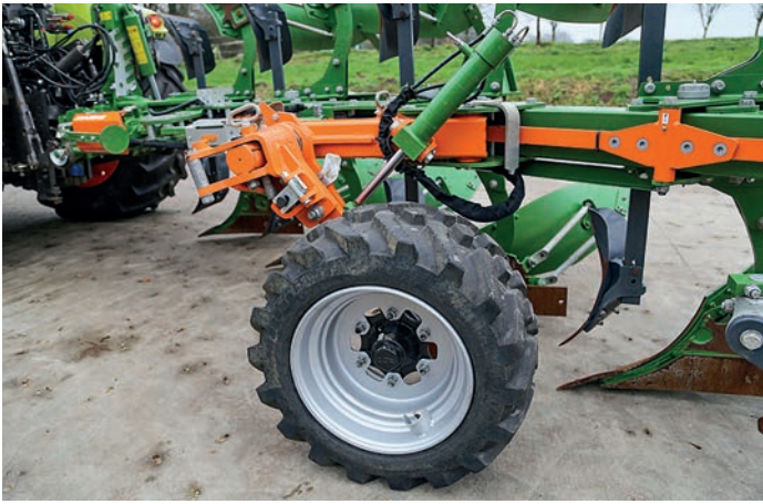
Combi wheel is available in hydraulic or, as shown here, mechanical versions. There are several tyre size options; we had the 360/45-17.5.
