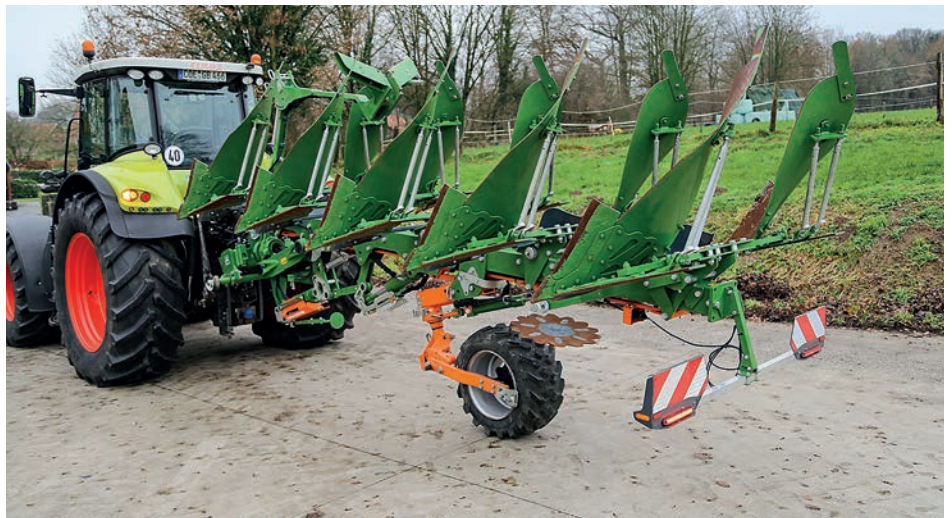
Just a few quick steps allow the combi wheel to share the plough's weight during transport, making the outfit much smoother on the road.
